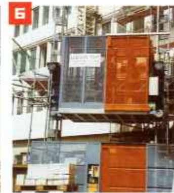
6 When the cage moves into the ground station, the cage door at the front is unlocked automatically and can be opened together with the sliding door of the ground station.
