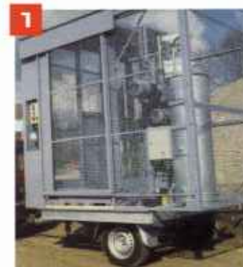
1 For the transport of the GEDA® 7P a uniaxial trailer is available. The loading/unloading is effected automatically by means of the hoist drive.
