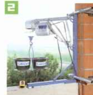
The window clamp is adjustable for wall thicknesses from 16-50 cm and is a practical fixing device for most window openings. In case of existing window posts the bearing points can be moved.
