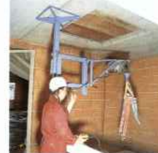
The floor to ceiling support also allows use under difficult conditions (e.g. in staircases).
