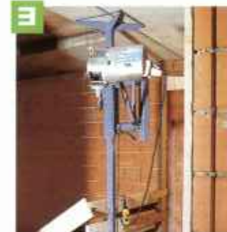
The floor to ceiling support can be extended from 230-325 cm. Due to an additional lockable swivel arm it has a very large working radius up to 155 cm and can even be used at very small windows (min. width approx. 70 cm) due to the two joints. The swivel arm can also be adjusted in height.
