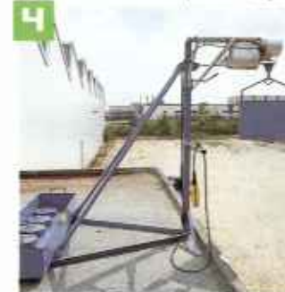
The free-standing tripod with ballast container for flat roofs and open floors can be disassembled for easy transport.
